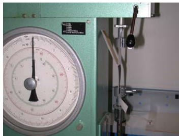
Tensile testing with clamped sample
