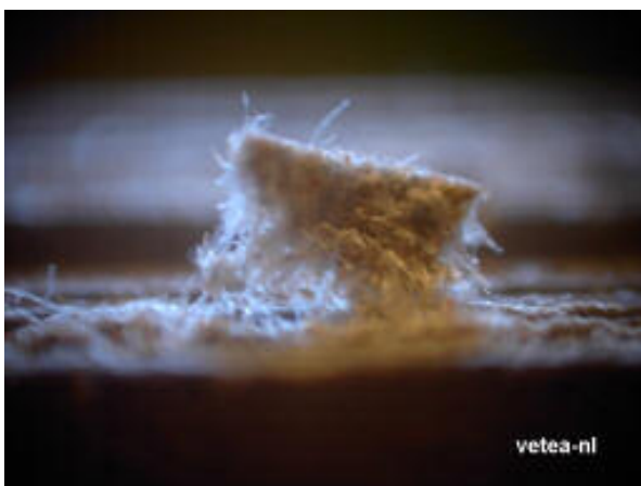
Figure 4: Fibre bundles pulled out of the face of the cut
