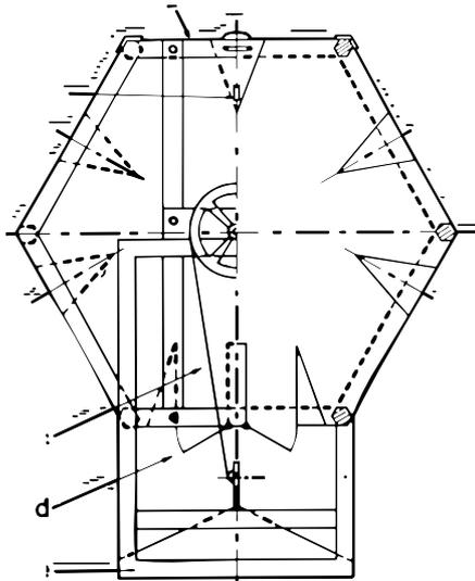
Figure 2. An example of a mixing drum for wood chips. The figure shows the end and a cross section of the drum, which is about 0,8 m high and 0,9 m in length.
